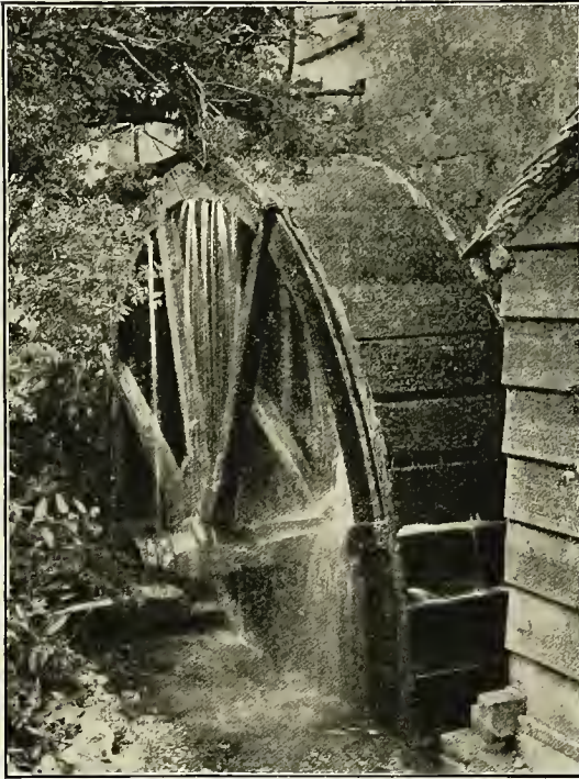
FIG. 48. — An old-fashioned water wheel used to give the power for grinding grain into flour in a grist mill.
